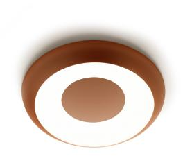
Ceiling or wall lighting fixture for interiors, with direct light emission.  $Turned\ steel\ structure\ in\ textured\ soft\ white,\ mat\ black,\ champagne,\ bronze,\ textured$ myrtle blue and textured natural terracotta polyacrylic paint. Aluminium wiring support plate with polyacrylate paint finish. Curved diffuser screen made of matt PMMA technopolymer. DALI/Push DIM driver available on request.
