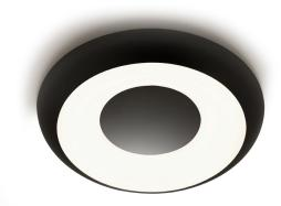
Ceiling or wall lighting fixture for interiors, with direct light emission. Turned steel structure in textured soft white, mat black, champagne, bronze, textured myrtle blue and textured natural terracotta polyacrylic paint. Aluminium wiring support plate with polyacrylate paint finish. Curved diffuser screen made of matt PMMA technopolymer. DALI/Push DIM driver available on request.
