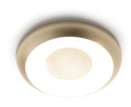
Ceiling or wall lighting fixture for interiors, with direct light emission.  $Turned\ steel\ structure\ in\ textured\ soft\ white,\ mat\ black,\ champagne,\ bronze,\ textured$ myrtle blue and textured natural terracotta polyacrylic paint. Aluminium wiring support plate with polyacrylate paint finish. Curved diffuser screen made of matt PMMA technopolymer. DALI/Push DIM driver available on request.
