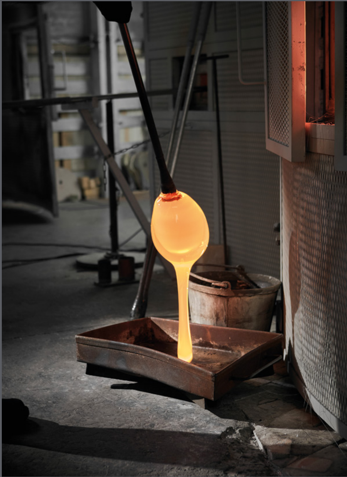
Molten glass comes out of the furnace at a temperature of around 1,100–1,200 °C; at this stage, it is in a viscous and malleable state, perfect for blowing or hot working.
