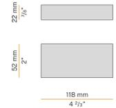
XM6-25 D/P MULTI LED driver, 11÷25,6W 200÷900mA, DALI/Push DIM dimmable.
