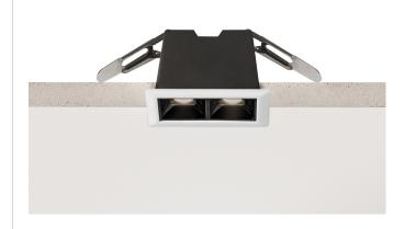
$Rectangular\ lighting\ fixture\ for\ ceiling\ built-in\ installation\ for\ interiors,\ with\ recessed$ direct light emission made of LED lens with 30à light beam.
