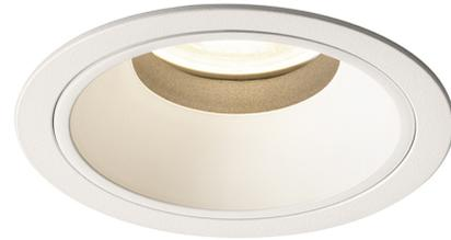
Lighting fixture for ceiling built-in installation for interiors, with direct light emission. Built-in structure for permanent false ceilings, in die-cast aluminium in white powder paint. Light source fastening ring in thermoplastic material. Reflector in thermoplastic material with white or mat black finish. Stainless steel spring clips for false ceiling fixing. Built-in hole dimension: Ø 75mm (Ø 3")
