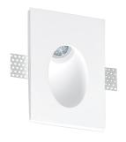
Lighting fixture for ceiling or wall built-in installation for interiors, with direct light emission. Total built-in plaster structure for masonry or plasterboard. Turned aluminium heat sink. Acrylic moulded lens. Light module closing frame in turned aluminium. Light source retaining spring clip in stainless steel. Fixing brackets in micro-perforated sheet metal. Recessed housing for masonry in galvanized sheet metal to be ordered separately. Built-in hole dimension: 110x175mm (4,3x6,9")
