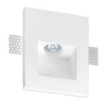
emission. Total built-in plaster structure for masonry or plasterboard. Turned aluminium heat sink. Acrylic moulded lens. Light module closing frame in turned aluminium. Light source retaining spring clip in stainless steel. Fixing brackets in micro-perforated sheet metal. Recessed housing for masonry in galvanized sheet metal to be ordered separately. Built-in hole dimension: 110x155mm (4,3x6,1")
