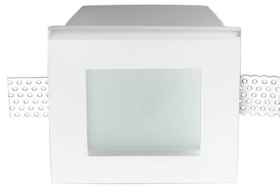
Lighting fixture for ceiling built-in installation for interiors, with direct light emission. Total built-in plaster structure for masonry or plasterboard. Light source retaining spring clip in stainless steel. Flat frosted glass diffuser. Fixing brackets in micro-perforated sheet metal. Recessed housing for masonry in galvanized sheet metal to be ordered separately. Built-in hole dimension: 125x125mm (4,9x4,9")
