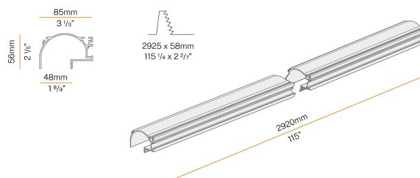
Modular profile for ceiling or wall built-in installation for interiors, with indirect light emission.
