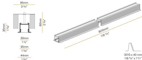
Modular profile for ceiling or wall built-in installation for interiors, with direct light emission.
