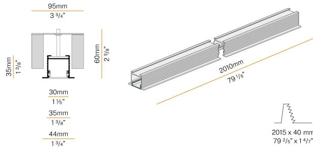
Modular profile for ceiling or wall built-in installation for interiors, with direct light emission.
