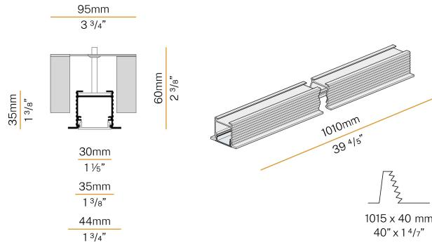
Modular profile for ceiling or wall built-in installation for interiors, with direct light emission.
