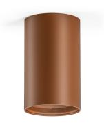
Ceiling lighting fixture for interiors, with direct light emission.  $\label{thm:extruded} \textbf{Extruded} \ \textbf{and} \ \textbf{milled} \ \textbf{aluminium} \ \textbf{structure,} \ \textbf{with} \ \textbf{polyacrylic} \ \textbf{paint} \ \textbf{finish} \ \textbf{in} \ \textbf{white,} \ \textbf{black,}$ bronze, mat brass, textured olive green or textured natural terracotta. Lens holder not included, to be purchased separately.
