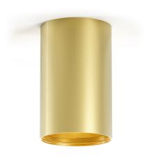
Ceiling lighting fixture for interiors, with direct light emission.  $\label{thm:extruded} \textbf{Extruded} \ \textbf{and} \ \textbf{milled} \ \textbf{aluminium} \ \textbf{structure,} \ \textbf{with} \ \textbf{polyacrylic} \ \textbf{paint} \ \textbf{finish} \ \textbf{in} \ \textbf{white,} \ \textbf{black,}$ bronze, mat brass, textured olive green or textured natural terracotta. Lens holder not included, to be purchased separately.
