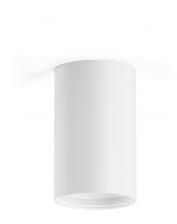
Ceiling lighting fixture for interiors, with direct light emission.  $\label{thm:extruded} \textbf{Extruded} \ \textbf{and} \ \textbf{milled} \ \textbf{aluminium} \ \textbf{structure,} \ \textbf{with} \ \textbf{polyacrylic} \ \textbf{paint} \ \textbf{finish} \ \textbf{in} \ \textbf{white,} \ \textbf{black,}$ bronze, mat brass, textured olive green or textured natural terracotta. Lens holder not included, to be purchased separately.
