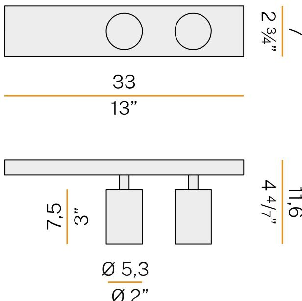
Ceiling or wall lighting fixture for interiors, with swivelling light beam.
