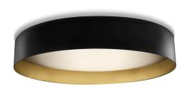
Ceiling or wall lighting fixture for interiors, with direct light emission.  $Turned\ aluminium\ structure\ in\ mat\ black\ and\ gold\ or\ white\ and\ gold\ polyacrylic\ paint.$ Pickled sheet metal wiring support plate in polyacrylic paint.  $\ \, \text{Moulded polycarbonate micro-prismatic diffuser}.$
