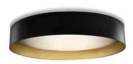
Ceiling or wall lighting fixture for interiors, with direct light emission.  $Turned\ aluminium\ structure\ in\ mat\ black\ and\ gold\ or\ white\ and\ gold\ polyacrylic\ paint.$ Pickled sheet metal wiring support plate in polyacrylic paint.  $\ \, \text{Moulded polycarbonate micro-prismatic diffuser}.$
