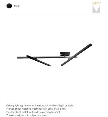
Structure with adjustable arms in pickled sheet metal in white or black polyacrylic paint. Aluminium dissipation plates in polyacrylic paint. Modelled polycarbonate screens with transparent finish.
