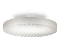
Ceiling or wall lighting fixture for interiors, with direct light emission. Die-cast aluminium structure in white polyacrylic paint. Diffuser screen made of frosted blown glass with matt white or smoke grey finish. Pickled sheet metal covering with ceiling fixing bracket in white polyacrylic paint.
