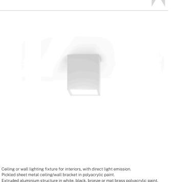
Pickled sheet metal ceiling/wall bracket in polyacrylic paint. Extruded aluminium structure in white, black, bronze or mat brass polyacrylic paint. Aluminium dissipation plate. Flat frosted glass diffuser. Pickled sheet metal frame in polyacrylic paint.
