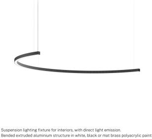
Suspension lighting fixture for interiors, with direct light emission. Bended extruded aluminium structure in white, black or mat brass polyacrylic paint. Extruded polycarbonate diffuser with opaline finish. Galvanized sheet metal end caps in polyacrylic paint. Suspension kit with griplocks and 5m (196,9") long steel cables. 5m (196,9") long power cable in transparent PVC. Power canopy with pickled sheet metal ceiling bracket and covering in white, black or mat brass polyacrylic paint.
