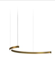
Suspension lighting fixture for interiors, with direct light emission. Bended extruded aluminium structure in white, black or mat brass polyacrylic paint. Extruded polycarbonate diffuser with opaline finish. Galvanized sheet metal end caps in polyacrylic paint. Suspension kit with griplocks and 2m (78,7") long steel cables. 2,2m (86,6") long power cable in transparent PVC. Power canopy with pickled sheet metal ceiling bracket and covering in white, black or mat brass polyacrylic paint.
