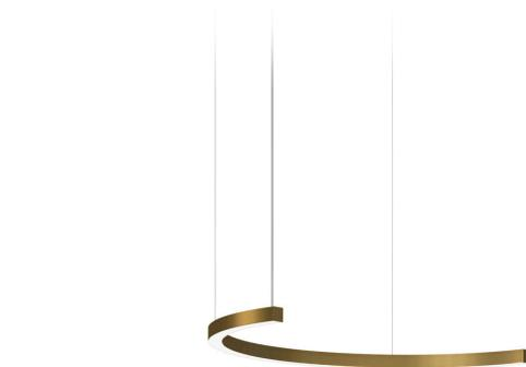
Suspension lighting fixture for interiors, with direct light emission. Bended extruded aluminium structure in white, black or mat brass polyacrylic paint. Extruded polycarbonate diffuser with opaline finish. Galvanized sheet metal end caps in polyacrylic paint. Suspension kit with griplocks and 2m (78,7") long steel cables. 2,2m (86,6") long power cable in transparent PVC. Power canopy with pickled sheet metal ceiling bracket and covering in white, black or mat brass polyacrylic paint.
