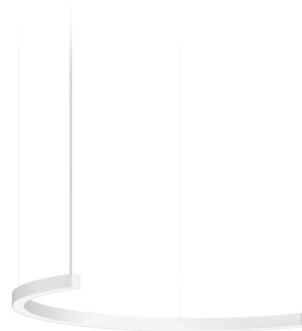
Suspension lighting fixture for interiors, with direct light emission. Banded extruded aluminium structure in white, black or mat brass polyacrylic paint. Extruded polycarbonate diffuser with opaline finish. Galvanized sheet metal end caps in polyacrylic paint. Suspension kit with griplocks and 2m (78,7") long steel cables. 2,2m (86,6") long power cable in transparent PVC. Power canopy with pickled sheet metal ceiling bracket and covering in white, black or mat brass polyacrylic paint.
