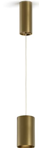
Suspension lighting fixture for interiors, with direct light emission. Extruded and milled aluminium structure, with polyacrylic paint finish in white, black, bronze, mat brass, textured olive green or textured natural terracotta. 3m (118,1") long suspension and coaxial power cable in transparent PVC. Power canopy with pickled sheet metal ceiling bracket and extruded aluminium covering with polyacrylic paint. Lens holder not included, to be purchased separately.
