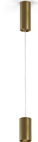
Suspension lighting fixture for interiors, with direct light emission. Extruded and milled aluminium structure, with polyacrylic paint finish in white, black, bronze, mat brass, textured olive green or textured natural terracotta. 3m (118,1") long suspension and coaxial power cable in transparent PVC. Power canopy with pickled sheet metal ceiling bracket and extruded aluminium covering with polyacrylic paint. Lens holder not included, to be purchased separately.
