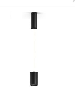
Suspension lighting fixture for interiors, with direct light emission. Extruded and milled aluminium structure, with polyacrylic paint finish in white, black, bronze, mat brass, textured olive green or textured natural terracotta. 3m (118,1") long suspension and coaxial power cable in transparent PVC. Power canopy with pickled sheet metal ceiling bracket and extruded aluminium covering with polyacrylic paint. Lens holder not included, to be purchased separately.
