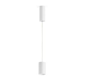
Suspension lighting fixture for interiors, with direct light emission. Extruded and milled aluminium structure, with polyacrylic paint finish in white, black, bronze, mat brass, textured olive green or textured natural terracotta. 3m (118,1") long suspension and coaxial power cable in transparent PVC. Power canopy with pickled sheet metal ceiling bracket and extruded aluminium covering with polyacrylic paint.
