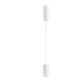
Suspension lighting fixture for interiors, with direct light emission. Extruded and milled aluminium structure, with polyacrylic paint finish in white, black, bronze, mat brass, textured olive green or textured natural terracotta. 3m (118,1") long suspension and coaxial power cable in transparent PVC. Power canopy with pickled sheet metal ceiling bracket and extruded aluminium covering with polyacrylic paint.
