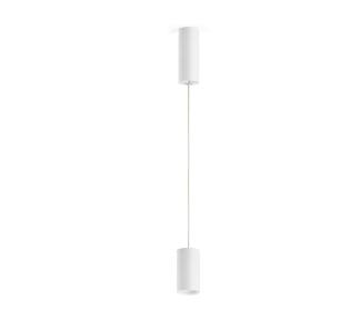
Suspension lighting fixture for interiors, with direct light emission. Extruded and milled aluminium structure, with polyacrylic paint finish in white, black, bronze, mat brass, textured olive green or textured natural terracotta. 3m (118,1") long suspension and coaxial power cable in transparent PVC. Power canopy with pickled sheet metal ceiling bracket and extruded aluminium covering with polyacrylic paint. Lens holder not included, to be purchased separately.
