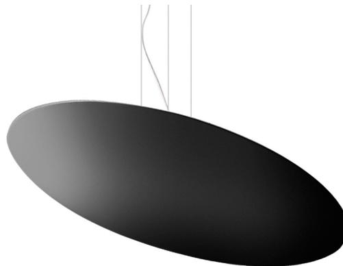
Suspension lighting fixture for interiors, with indirect light emission. Aluminium and pickled sheet metal structure in polyacrylic paint. Turned aluminium reflector in white or black polyacrylic paint or with gold leaf coating. Moulded acrylic diffuser with mat finish. 2m (78,7") long steel suspension cables. 2,2m (86,6") long power cable in transparent PVC. Power canopy with pickled sheet metal case in white or black polyacrylic paint or with gold leaf coating.
