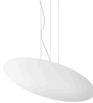
Suspension lighting fixture for interiors, with indirect light emission. Aluminium and pickled sheet metal structure in polyacrylic paint. Turned aluminium reflector in white or black polyacrylic paint or with gold leaf coating. Moulded acrylic diffuser with mat finish. 2m (78,7") long steel suspension cables. 2,2m (86,6") long power cable in transparent PVC. Power canopy with pickled sheet metal case in white or black polyacrylic paint or with gold leaf coating.
