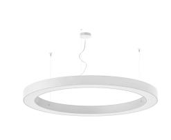
Pickled sheet metal structure in polyacrylic paint. Aluminium dissipation plates. Pickled sheet metal covers in white, black or bronze polyacrylic paint, or with gold leaf coating. Diffuser in modelled polycarbonate with opaline finish. Suspension kit with griplocks and 5m (196,9") long steel cables. 5m (196,9") long power cable in transparent PVC.
