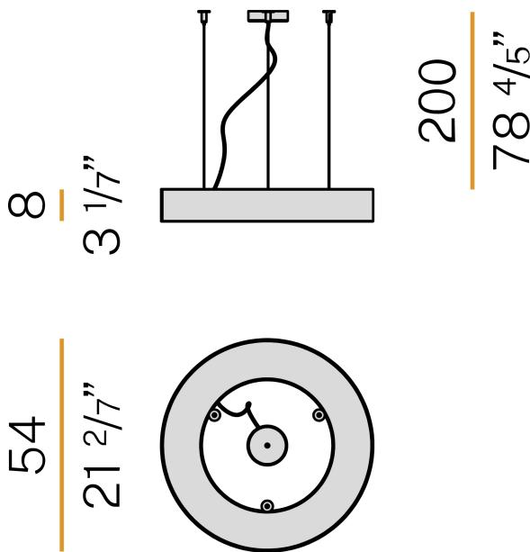
Suspension lighting fixture for interiors, with direct light emission.
