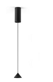
Suspension lighting fixture for interiors, with direct light emission.  $\label{eq:decomposition} \mbox{Die-cast aluminium head with polyacrylic paint finish in mat black or bronze.}$ Turned aluminium end plate with polyacrylic paint in mat black or bronze. Black PVC coaxial suspension and power cable 3m (118.1") long. Feeding canopy with ceiling mounting bracket in pickled sheet metal and extruded aluminium housing with polyacrylic paint finish in mat black or bronze. \\
