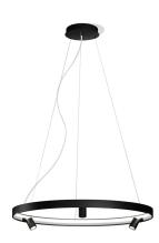
Suspension lighting fixture for interiors, with direct and indirect light emission and swivelling accent light. Bended extruded aluminium structure in white, black, bronze, mat brass or titanium polyacrylic paint. Extruded polycarbonate diffuser with opaline finish. Die-cast aluminium joints in polyacrylic paint. Die-cast aluminium projectors rotating on two axes in polyacrylic paint. Reflectors in thermoplastic material with chrome plated finish. Textured glass screens.
