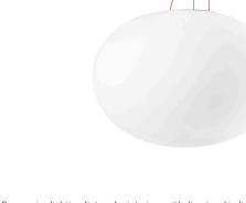
Suspension lighting fixture for interiors, with direct and indirect light emission. Pressed pickled sheet metal structure in white polyacrylic paint. Extruded aluminium heat sink. Diffuser in mat white blown glass. 2m (78,7") long steel suspension cable. 2m (78,7") long double power cable in red Teflon. Power canopy with galvanized sheet metal ceiling bracket and pickled sheet metal covering in white polyacrylic paint.
