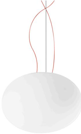
Suspension lighting fixture for interiors, with direct and indirect light emission. Pressed pickled sheet metal structure in white polyacrylic paint. Extruded aluminium heat sink. Diffuser in mat white blown glass. 2m (78,7") long steel suspension cable. 2m (78,7") long double power cable in red Teflon. Power canopy with galvanized sheet metal ceiling bracket and pickled sheet metal covering in white polyacrylic paint.
