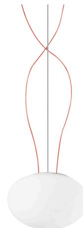
Suspension lighting fixture for interiors, with direct and indirect light emission. Pressed pickled sheet metal structure in white polyacrylic paint. Aluminium dissipation plate. Diffuser in mat white blown glass. 2m (78,7") long steel suspension cable. 2m (78,7") long double power cable in red Teflon. Power canopy with galvanized sheet metal ceiling bracket and pickled sheet metal covering in white polyacrylic paint.
