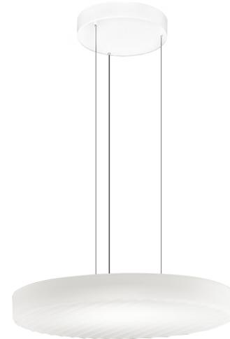
Suspension lighting fixture for interiors, with direct light emission. Die-cast aluminium structure in black or white polyacrylic paint. Diffuser screen made of frosted blown glass with matt white or smoke grey finish. 2m (78,7") long steel suspension cables. 2,2m (86,6") long power cable in transparent PVC. Power canopy with metal ceiling bracket and pickled sheet metal covering in white or black polyacrylic paint.
