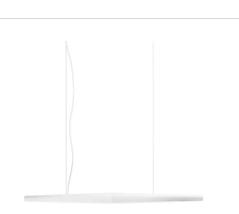
Suspension lighting fixture for interiors, with direct light emission. Machined aluminium structure in white or black polyacrylic paint. Anodized extruded aluminium heat sink. Extruded polycarbonate diffuser with opaline finish. Suspension kit with griplocks and 2m (78,7") long steel cables. 2m (78,7") long power cable in transparent PVC. Power canopy with galvanized sheet metal ceiling bracket and pickled sheet metal covering in white or black polyacrylic paint.
