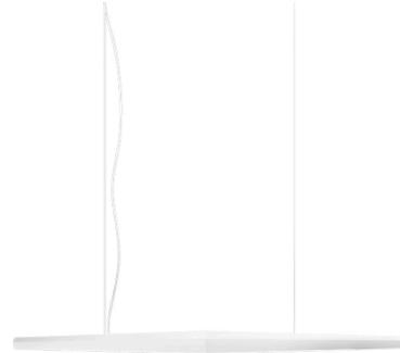
Suspension lighting fixture for interiors, with direct light emission. Machined aluminium structure in white or black polyacrylic paint. Anodized extruded aluminium heat sink. Extruded polycarbonate diffuser with opaline finish. Suspension kit with griplocks and 2m (78,7") long steel cables. 2m (78,7") long power cable in transparent PVC. Power canopy with galvanized sheet metal ceiling bracket and pickled sheet metal covering in white or black polyacrylic paint.
