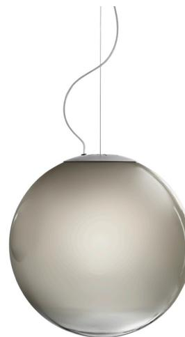
Suspension lighting fixture for interiors, with direct and indirect light emission. Pickled sheet metal structure in titanium polyacrylic paint. Diffuser in hand-crafted blown glass with white or smoke-grey shaded effect. 2m (78,7") long steel suspension cable. 2m (78,7") long power cable in transparent PVC. Power canopy with galvanized sheet metal ceiling bracket and pickled sheet metal covering in titanium polyacrylic paint.
