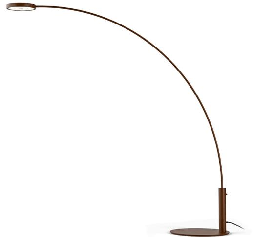
Floor lighting fixture for exteriors, with direct or indirect light emission. Circular bearing base in metal, with polyacrylic paint. Calendered steel tube stem, with polyacrylic paint. Die-cast aluminum emitting head with polyacrylic paint in corten, olive textured green, soft textured white and micaceous grey. UV technology screen-printed diffuser, made of opal polycarbonate.
