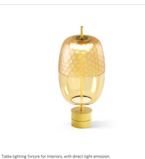
Aluminium frame with polyacrylic paint finish in mat black or mat brass. Diffuser screen in acrylic material with satin finish. Handmade and hand-ground blown glass in bronze colour. Steel closing plate with polyacrylic paint finish. Metal base with polyacrylic paint in mat black or mat brass finish, with integrated dimmer button. Supplied complete with black fabric power cable and plug adapter.
