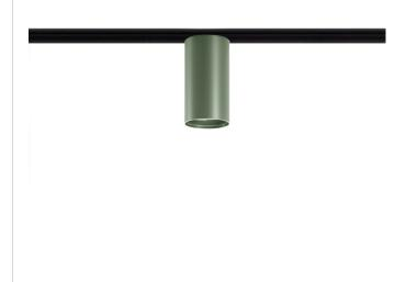
Ceiling lighting fixture for interiors, with direct light emission.  $\label{thm:extruded} \textbf{Extruded} \ \text{and} \ \textbf{milled} \ \textbf{aluminium} \ \textbf{structure,} \ \textbf{with} \ \textbf{polyacrylic} \ \textbf{paint} \ \textbf{finish} \ \textbf{in} \ \textbf{white,} \ \textbf{black,}$ bronze, mat brass, textured olive green or textured natural terracotta.
