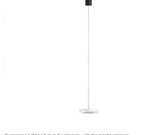
Suspension lighting fixture for interiors, with direct light emission. Die-cast aluminium structure in white, black, bronze or mat brass polyacrylic paint. Modelled acrylic diffuser with mat finish. Aluminium closing disk in polyacrylic paint. Suspension kit with rod in brass tube in polyacrylic paint. 3m (118,1") long suspension and coaxial power cable in transparent PVC. Black power supply canopy with 48V track adaptor for the Street track series.
