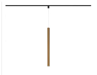
Suspension lighting fixture for interiors, with direct light emission. Extruded aluminium structure in white, mat black, bronze or mat brass polyacrylic paint. Modelled polycarbonate diffuser with opaline finish. Turned brass end cap in polyacrylic paint. 3m (118,1") long suspension and power cable in transparent PVC.
