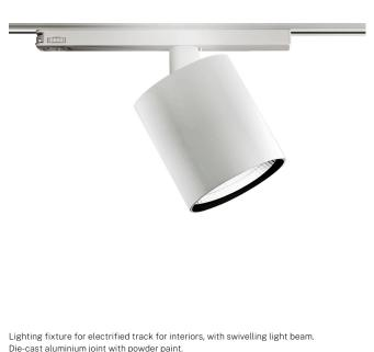
Lighting fixture for electrified track for interiors, with swiveling light beam. Die-cast aluminium joint with powder paint. Die-cast aluminium structure rotating on two axes in white or black powder paint. Reflector in thermoplastic material with chrome plated finish. Anti-glare snoot in black thermoplastic material.
